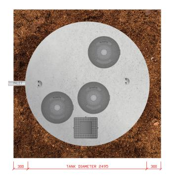
The lid of the tank should be 100-150mm above finished ground level, so be sure to allow for any topsoil or turf that may be laid around the tank after the tank installation.
